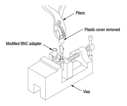
Figure 7: Removing plastic covers from binding posts
